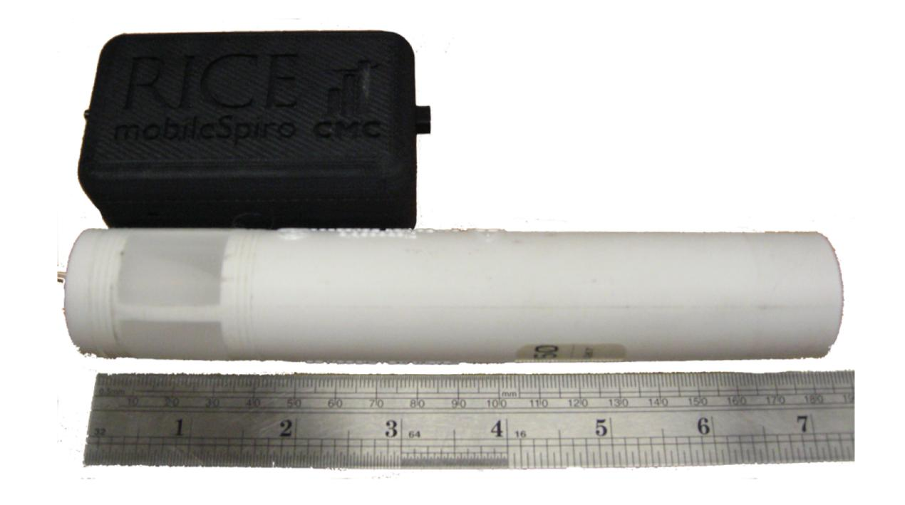
mobileSpiro is a custom spirometer which gives us access to raw data values during spirometer maneuvers. This allows us to customize the game based on the data.
